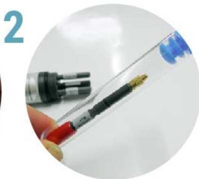
2 Remove the sensor from the container and remove the red sensor cap.
