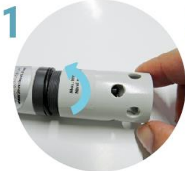
1 Unscrew the protection of the Multi Ion probe.
