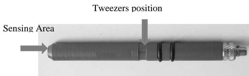
Place the electrode applying a small rotation pressure until the "o" ring are completely placed on the probe and the pin is connected.
