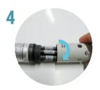
Screw on the protection without touching the tip of the sensors.
