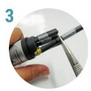
Hold the sensor with the tweezers and insert the desired channel through the end of the gold connector.
